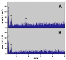
Fig. 5. Spectrographs of Si-treated (A) and not treated (B, control) leaf margins. The spectrograph was able to detect Si in significant amounts in the Si-treated samples (above background levels), but was not able to detect Si in the control plants.
