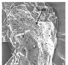
Fig. 4. A scale on a serration of a New Guinea impatiens with the corresponding X-ray map of the Si deposition overlaid on the photograph. There is a stronger concentration of Si, as indicated by the dot map, in the area occupied by the scale indicating Si is localized in the scales.
